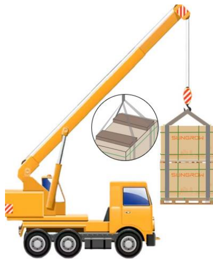
Fig. 3 Diagrammatic sketch of lifting the Modules
