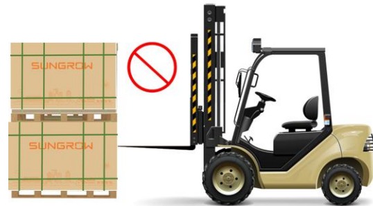
Fig. 5 Do not touch the box body with forks
