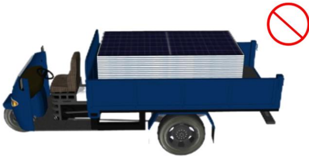
Fig. 6 Do not use tricycles to transport the Modules
